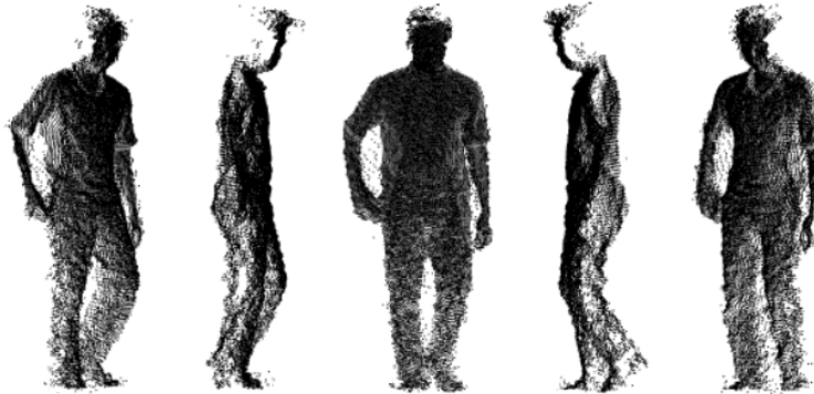
Figure 1: Example of a point cloud obtained in our setup for an application of gait analysis.
