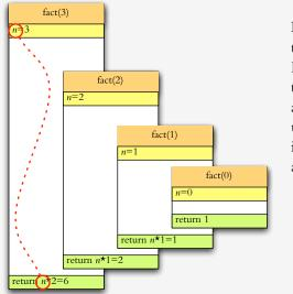
During the execution, the program needs to recover the context (e.g., parameter n) after returning from a recursive call. It is impossible to predict the depth of the recursion at compiletime. Memory for local variables and parameters needs to be allocated at run-time. Typically, the run-time environment uses a **call stack**. Whenever a procedure is activated, a block is allocated on the call stack to store the parameters, local variables, and the return address.
