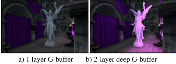
Figure 14: Radiosity in Sponza . A second layer captures reflection off the barely-seen purple banners on the right.
