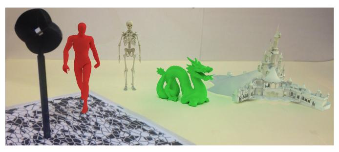
Figure 1: Augmented reality scene rendered in real-time on an iPad 3 using captured shading from a 3D printed shading probe (left).
