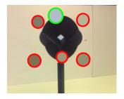
**Figure 3:** The left image is a photograph of a 3D printed 6D shading probe. The right image shows all the six acquired shading samples from the probe. Each overlaid colored disk represents such a sample, with its center showing the actual shading value and its outline indicating current from-camera visibility.
