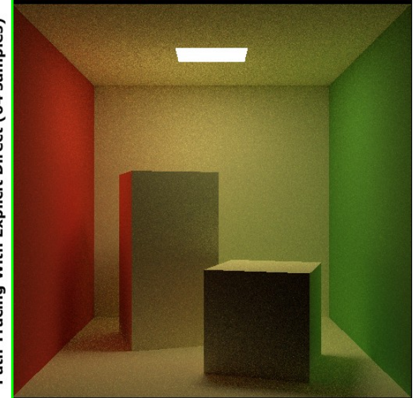
Path Tracing With Explicit Direct (64 samples)
