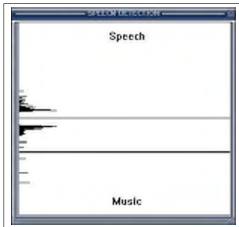
Figure 7: A Winamp plugin version of our model. The long thin horizontal line displays the decision boundary between Speech (top) and Music (bottom). The long thick horizontal line displays the decision of the model, with vertical position proportional to confidence. Here, for example, the model is moderately confident that the stream is Music (in this case, a correct prediction). The shorter horizontal lines on the left provide a histogram of the decisions and confidence ratings of the weak learners. See text for details.
