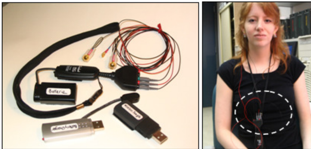
Fig. 1. Pendant EEG on the left and the Learner wearing it on the right
