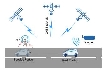
FIGURE 6. Illustration of a GNSS spoofing attack.
