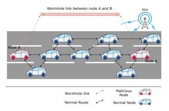
FIGURE 8. Wormhole Attack in VANET.
