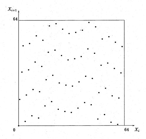
Figure 1: The pairs  $(X_i, X_{i+1})$ , for i = 1, ..., 63, produced by the Tausworthe sequence  $X_i = \sum_{j=1}^6 a_{4i+j} 2^{6-j}$ , where  $\{a_j\}$  follows the recurrence  $a_j = (a_{j-5} + a_{j-6}) \mod 2$ .
