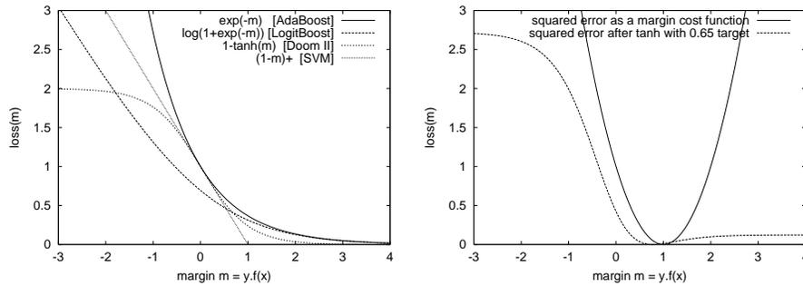
Figure 1: *Boosting and SVM margin loss functions (left) vs. traditional loss functions (right) viewed as functions of the margin. Interestingly the last-born of the margin motivated loss functions (used in Doom II) is similar to the traditional squared error after tanh.*
