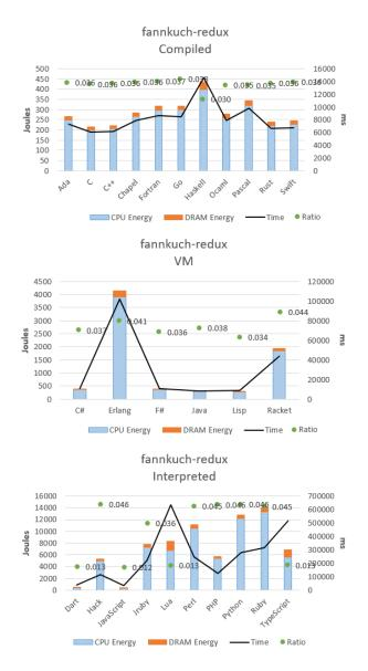
Figure 2: Energy and time graphical data for fannkuch-redux
