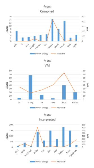
Figure 6: Energy and memory graphical data for fasta
