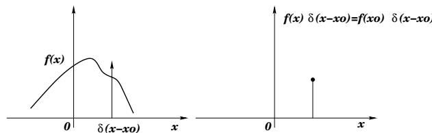
$$\begin{aligned} f(x) * \delta &= f(x) \\ f(x) * \delta_{x_0} &= f(x - x_0) \\ \mathcal{F}[f(x) \exp(2j\pi\nu_0 x)] &= F(\nu - \nu_0) \end{aligned}$$
