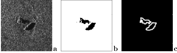
Figure 4: (a) Sonar image. (b) Associated Markovian two-class segmentation. (c) Edge potential field with \sigma = 1 .
