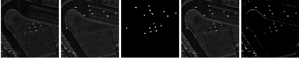
Fig. 3. Experimental results on SAR airborne dataset; From left to right; image acquired at time t_1 and t_2 , ground truth; Second row: similarity feature map, final (changed/unchanged) binary segmentation result obtained by our approach.
