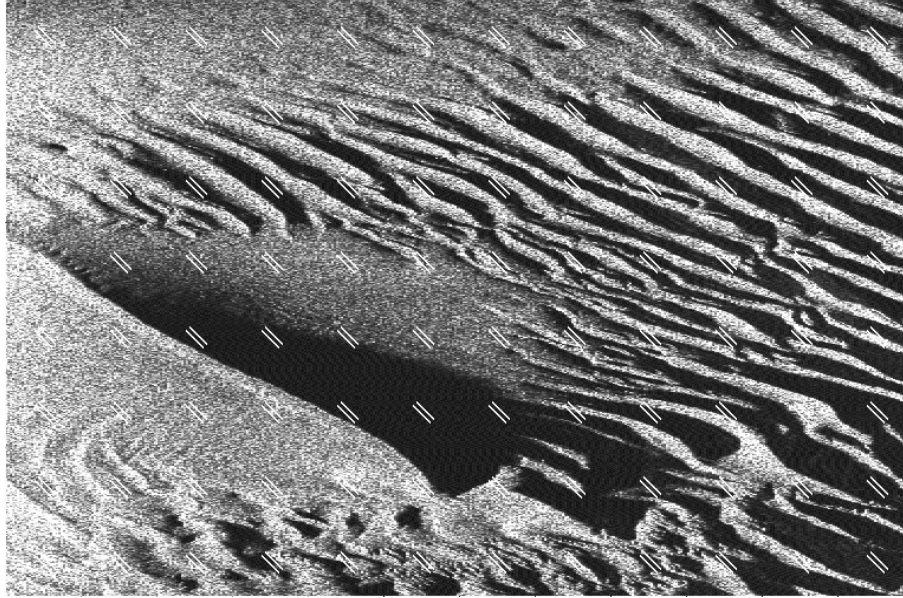
Figure 6: Original sidescan sonar image of an area composed by dunes (display convention: square with two parallel lines) and classification results obtained with our scheme. In this example, the adopted multi-scale classification strategy allows to efficiently recognize large cast shadow shapes created by dunes of sand and to obtain a right classification and segmentation map.
