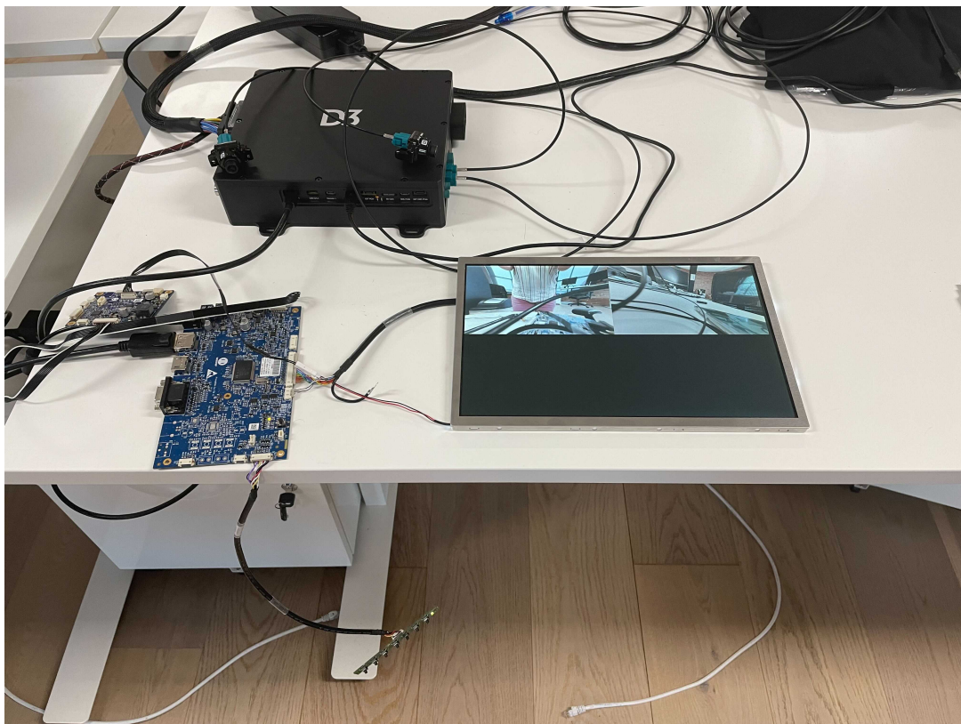
Figure 5.1: TDA4 platforms with cameras
