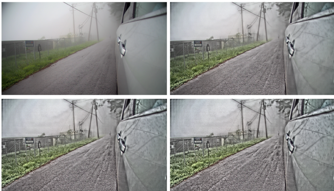
Figure 3.8: Original image and its enhancements by CLAHE, grid size: 32 \times 32 , clip limits: 4,8,12
