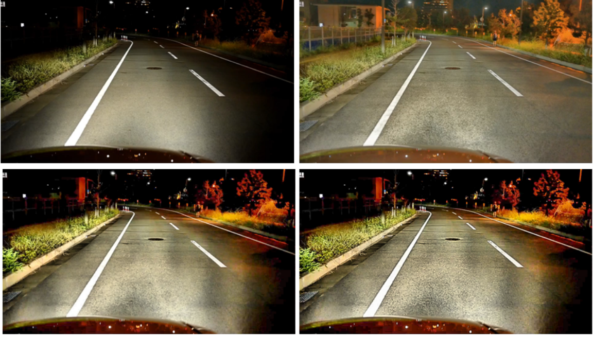
Figure 3.12: Homomorphic filtering result
