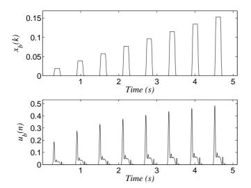
Fig. 3. Illustration of the dynamic compression and weighted differentiation steps for an artificial signal. Upper panel shows  $x_b(k)$  and the lower panel shows  $u_b(n)$ .
