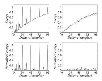
Fig. 4. Resonator energies for an impulse train with a period-length of 24 samples (left) and for white noise (right). Upper panels show the energies  $\hat{r}_c(\tau,n)$  and the lower panels normalized energies  $s_c(\tau,n)$ .
