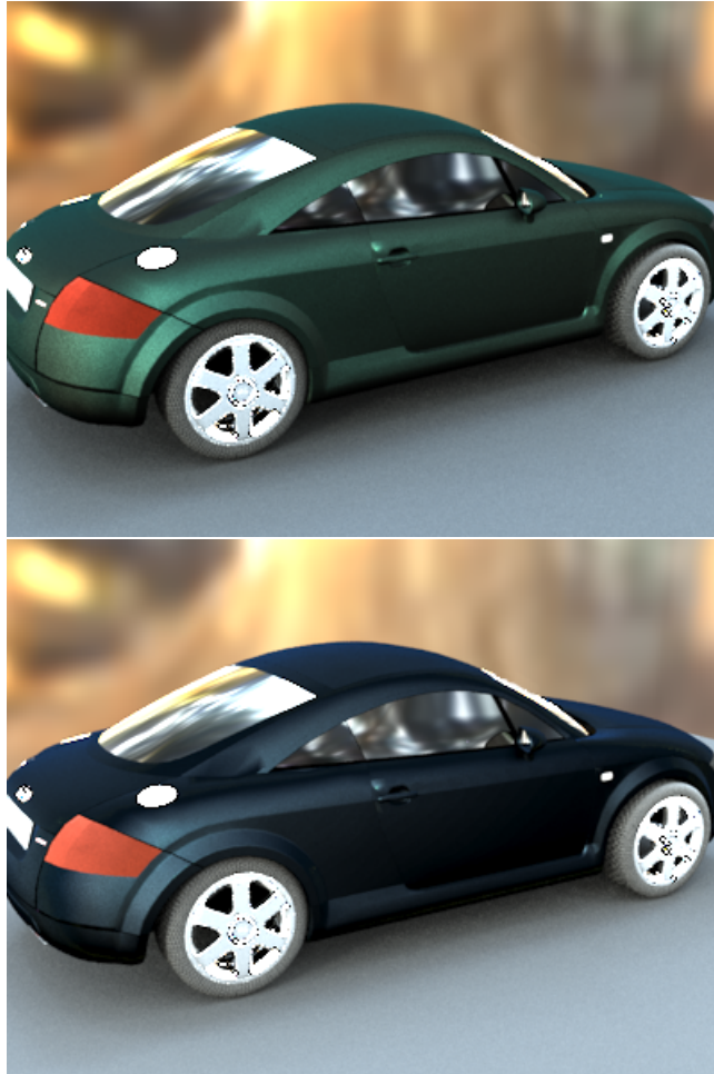
Figure 3.13: The Audi-TT model rendered with acquired BRDFs of 2 different paint samples. The BRDFs were acquired using 25 4^{th} order basis functions as defined in this chapter, and then rendered with a basis transformation into spherical harmonics. Top: Metallic teal automotive paint. Bottom: Krylon TM true blue paint. In each case, the time taken for the entire BRDF measurement process including data capture and re-projection into the spherical harmonic basis was about one minute.
