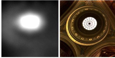
Figure 6.8: Factorization of an HDR photograph for the LED-based display. Left: LED contribution as a result of convolving LED values with the LED point spread function. Right: edge enhanced LCD panel image that corrects for the blurriness of the LED image.
