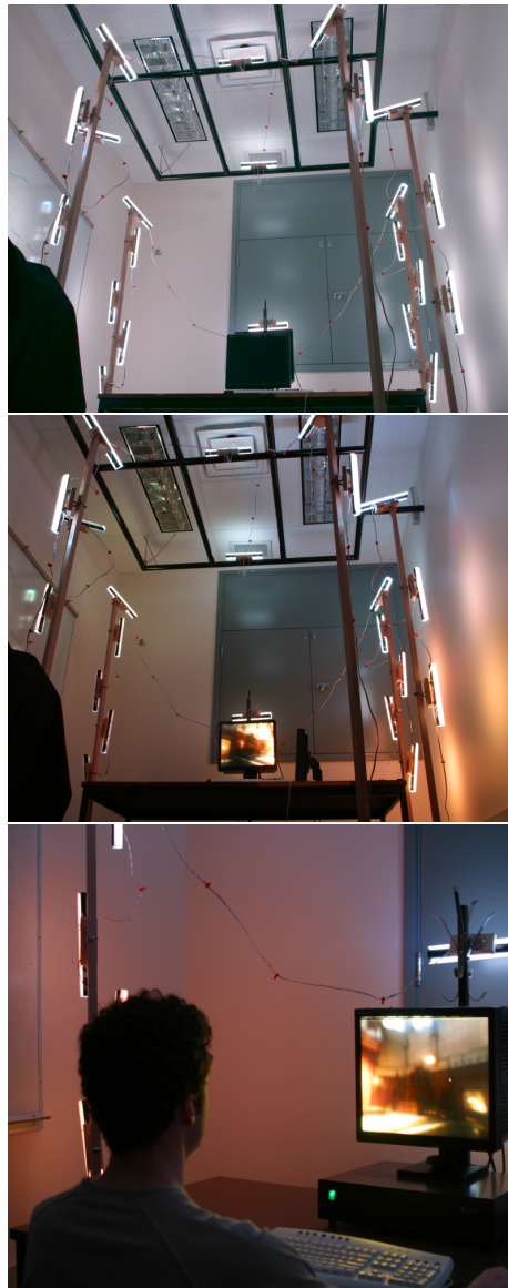
Figure 7.11: Top: photograph of the room housing our system, with all lights switched on. Center: illumination programmed to resemble the Grace Cathedral environment. Bottom: A user viewing the Grace Cathedral environment on an HDR display in a room illuminated by our system. Note how the room illumination is consistent with the virtual environment shown on the screen.
