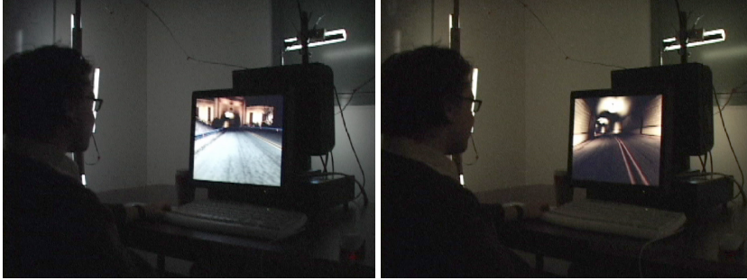
Figure 7.5: Left: room lighting corresponding to a passing street lamp on the left side in the driving game NFS Underground 2. Right: lighting corresponding to overhead lights and lights on the walls inside a tunnel in the game.
