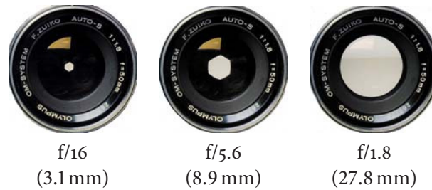
Figure 1.4: Non-circular variation in aperture for a real 50 mm SLR lens.
