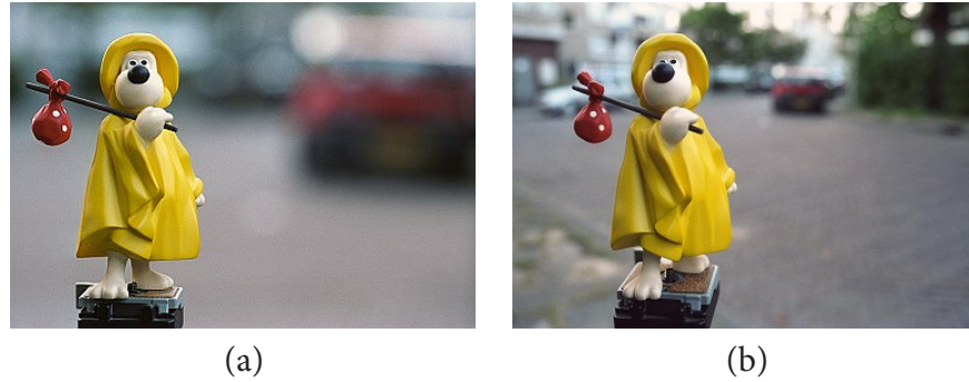
Figure 2.2: Changing the zoom setting from (a) telephoto (100 mm), to (b) wide-angle (28 mm), but moving the camera to keep the figurine roughly constant-size in the image. With this compensation the depth of field remains nearly constant, despite popular belief to the contrary. Note how flattened perspective in the telephoto case causes the background to be relatively magnified. © dpreview.com
