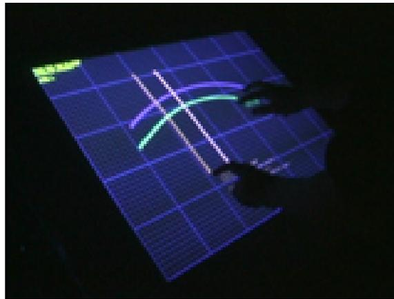
Figure 2.3: Multi-point interaction based on Frustrated Total Internal Reflectance.
