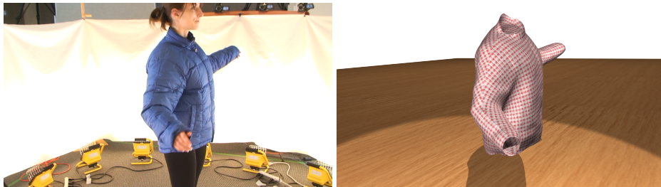
Figure 3.17: Capture result for a long-sleeve nylon-shell down jacket
