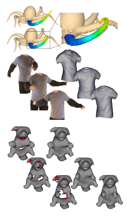
Figure 1.5: Results from this thesis. Top: Deformation of an octopus tentacle using the deformation technique presented in chapter 2. Middle: Detailed garment reconstruction result using a reconstruction method presented in chapters 3 and 4. Video stream (left) and reconstructed geometry (right). Bottom: Reconstruction of geometry and motion of a deformable hand-puppet using an acquisition technique presented in chapter 5. Initial reconstruction (left), final result (right)
