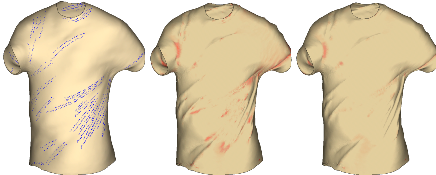
Figure 4.6: Deformation: (left) anchor triangles (fold edges projected to input garment); (center) vertex positioning result; (right) garment after stretch reduction. The coloring (center, right) shows per-triangle stretch. The iterations reduce the maximal per-triangle stretch from 8% to 4%
