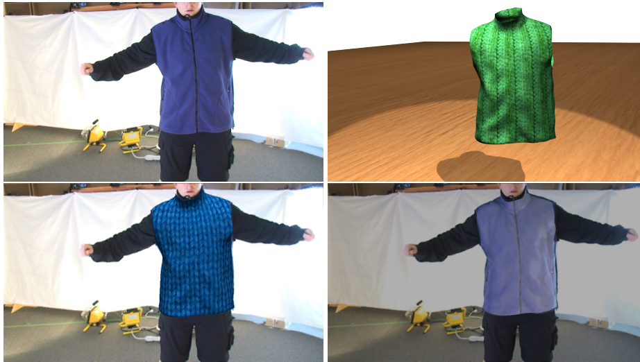
Figure 3.13: Capture results for a fleece vest. From top-left to bottom-right: one input frame, captured geometry, vest is replaced in the original image, the scene is augmented by adding a light source and making the vest more specular
