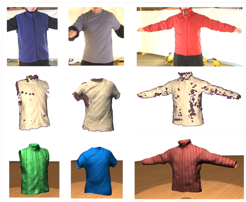
Figure 3.4: Result of multiview reconstruction for different garments (middle row). One of the sixteen input images is shown above each result, and the final reconstruction after parameterization and completion is shown below.
