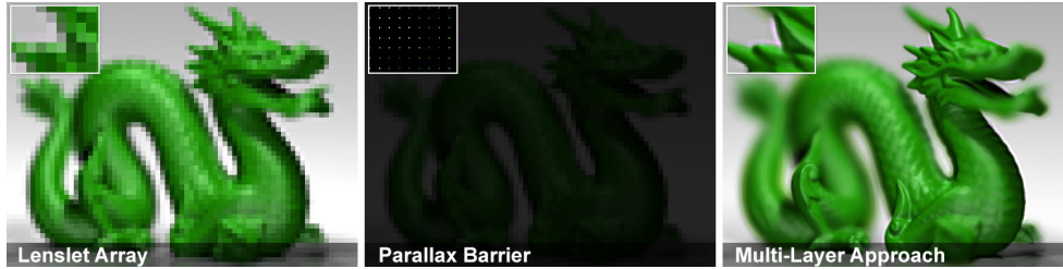
Figure 3.14: Benefits of multi-layer automultiscopic displays. Simulated views of the “dragon” are shown, from left to right, using integral imaging, parallax barriers, and the proposed multi-layer approach. Display parameters are selected to allow 7 \times 7 views, leading to a similar reduction in resolution for conventional methods. Compared to parallax barriers, the multi-layer approach is 49 times brighter and exceeds the resolution of both methods by a similar factor.
