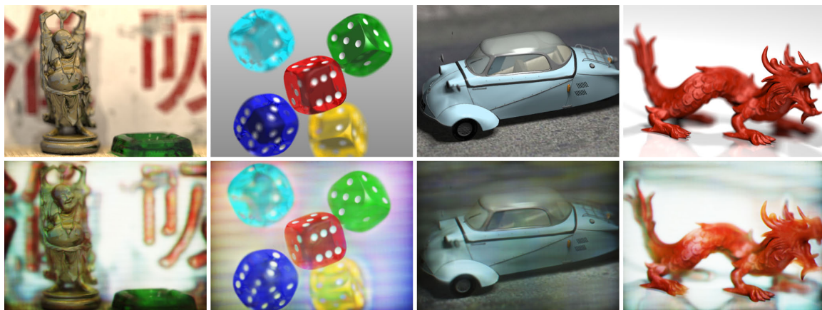
Figure 4.6: Polarization field display using the multi-layer prototype. The central views (perpendicular to the display) for the “Buddha”, “dice”, “car”, and “red dragon” scenes. Target views are compared to photographs of the prototype on the top and bottom, respectively. Colour imagery is obtained by combining three photographs taken while varying the colour channel displayed by the monochrome panels. Section 4.4 quantitatively assesses performance and artifacts.
