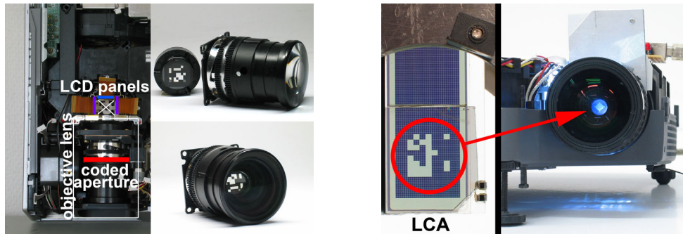
Figure 5.4: Two prototypes fabricated by Max Grosse at the Bauhaus University Weimar: a static attenuation mask integrated into the aperture plane of a projector improves digital defocus compensation through inverse filtering (left). Replacing the aperture with a transparent liquid crystal array allows dynamic attenuation mask patterns to be encoded (right). We compute the adaptive patterns by optimizing for light throughput while preserving spatial frequencies that are perceivable by a human observer. Both approaches significantly improve depth-of-field through inverse light filtering when compared to circular aperture stops. While static coded apertures are easier to realize and less expensive, adaptive coded apertures are more efficient.
