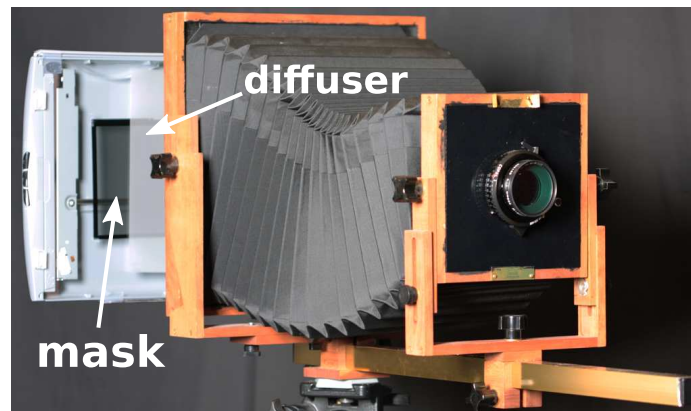
Figure 10.4: Our prototype is a large format high-resolution scanner camera. The filters are mounted under a diffuser on the scanner's glass plate.
