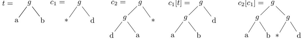
Figure 1: Examples of trees ( $t, c_1[t] \in \mathfrak{T}_{\mathcal{F}}$ ) and contexts ( $c_1, c_2, c_2[c_1] \in \mathfrak{C}_{\mathcal{F}}$ ) on the ranked alphabet  $\mathcal{F} = \mathcal{F}_0 \cup \mathcal{F}_2$  where  $\mathcal{F}_0 = \{a, b, d\}$  and  $\mathcal{F}_2 = \{g\}$ . With our notations:  $c_1[t] = g(g(a, b), d)$ ,  $|c_1[t]| = 5$ ,  $\text{depth}(c_1[t]) = 2$ ,  $\langle t \rangle = ab$ ,  $\text{drop}(c_2[c_1]) = 2$
