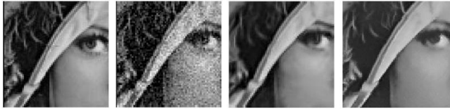
Fig. 4. Comparison between non-local effect and our acceleration result. From left to right, original image, noised image, the result of non-local [4] (MSE 68) and our result (MSE 81).
