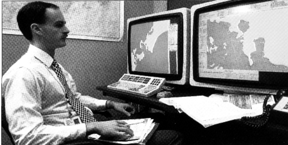
Figure 2: Photo from the article “Navigating Close to Shore” by Dave Dooling (“IEEE Spectrum”, Dec. 1994), © 1994 IEEE, photo by Intergraph Corp. 92° viewing angle. The two monitors have the same size. But the left one appears to be wider (misperception).
